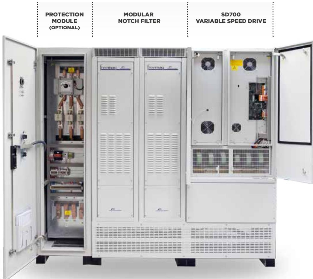
The passive filters are usually LC filters designed specifically to filter the 5<sup>th</sup> and 7<sup>th</sup> harmonic for a specific grid configuration and impedance  $Z_g$ . If the grid impedance is modified due to the introduction of new loads or motors, the filtering features are modified and may cause a resonance effect in the worst case.
